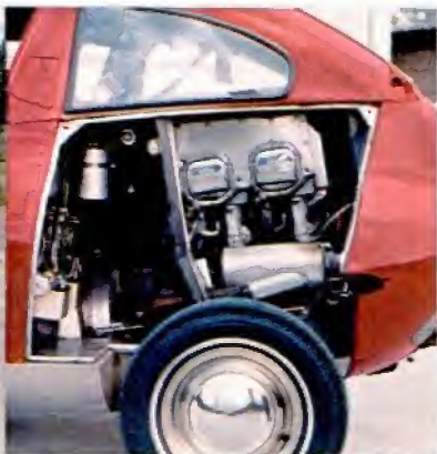
LYCOMING AIRCRAFT ENGINE with special ignition and cooling systems powers both car and plane
